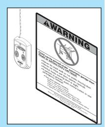
FIG. 3-5 Mounting Entrapment warning label.
